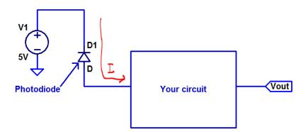
3. Re-design the circuit in problem 2 so that the output varies from −1 V to −2 V, that is, an input of 0 uA gives −1 V output while an input of 1 uA gives an output of −2 V. Note that you can accomplish this design using the design in problem 2 with an added voltage source (only). Simulate your design as done in problem 2. (2 points)
