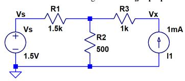
3. Find the voltage Vx in the circuit seen below. Then find the Thevenin equivalent circuit, with R2 removed, at the terminals marked by dots. Show that your Thevenin circuit is correct by comparing the value you calculated for Vx to the one you get when you put R2 across the terminals of your Thevenin equivalent. (20 points)
