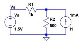
2. Find Vx in the following circuit using superposition. (10 points)
