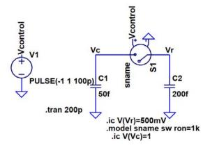
2. Plot the output of the following circuit from a time 0 to 10 ms. Assume the capacitor is initially discharged (both sides are at ground). Show your hand calculations for credit. Verify your plot with LTspice. (3 points)
