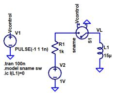
Note that the initial current through the inductor is zero.
