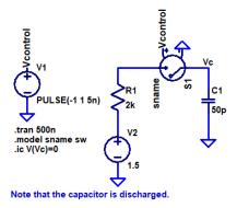
3. Write the equations describing the voltage across the capacitor, Vc, in the following circuit for both the rising and falling edges of the input pulse. Again, use LTspice to verify your answer. (3 points)
