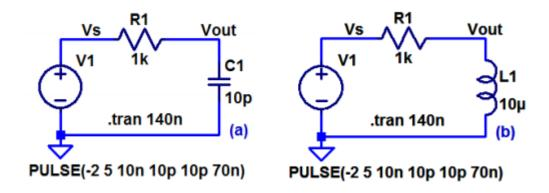
7. Plot the output of the following circuit from a time 0 to 5 ms. Assume that the capacitor is initially discharged (both sides are at 0 V). Ensure you show how you calculate Vout. (10 points)
