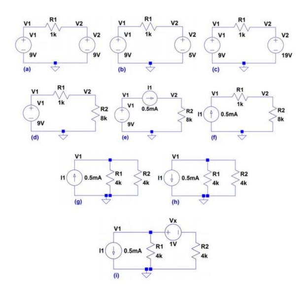
2. Using superposition show how to find Vx in each of the following circuits. Show your work for credit. (10 points)
