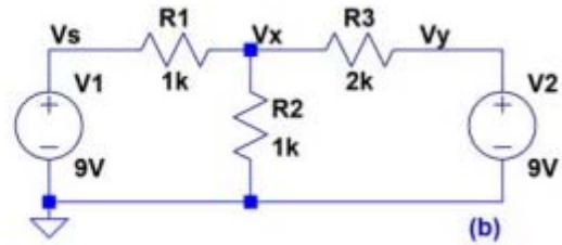
4. Find the Thevenin and Norton equivalent circuits between  $V_x$  and ground with  $R_2$  removed in the following circuits. Show your work for credit. (10 points)
