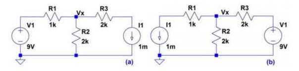
3. Find the voltages and currents in each of the following circuits using mesh analysis. Show your work for credit. (10 points)
