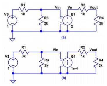
6. Write the equations and sketch along with the input pulse (on the same plot), for each of the input pulse's transitions, for the output of each of the following circuits. (10 points)
