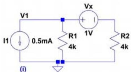
2. Using superposition show how to find  $V_x$  in each of the following circuits. Show your work for credit. (10 points)
