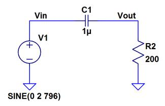
9. For the circuit in problem 8 determine, and sketch, the magnitude and phase responses of Vout/Vin. Your plots should be dB on the y-axis and log of frequency on the x-axis. (10 points)
