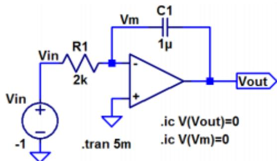
8. Using phasor analysis sketch  $V_{out}$  and  $V_{in}$ , on the same plot, for the following circuit. Show your work (how you calculate the magnitude and phase shift of the output) for credit. Note that the input's peak voltage is 2 V. (10 points)
