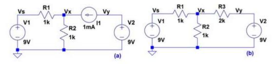
4. Find the Thevenin and Norton equivalent circuits between Vx and ground with R2 removed in the following circuits. Show your work for credit. (10 points)
