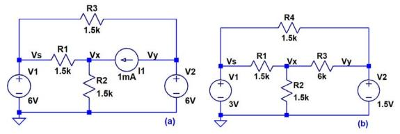
3. For the circuits in problem 2 find the Thevenin and Norton equivalent circuits from Vx to ground without R2 in the circuit. Show, with R2 back in the circuit, that you get the same value for Vx that you calculated in problem 2. Verify your Thevenin and Norton circuits are correct using LTspice. (4 points)
