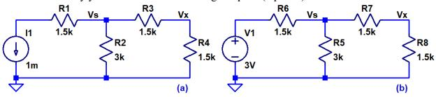
3. Using superposition show how to find Vx in the following circuits. Verify your hand calculations using LTspice. (6 points)
