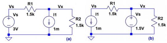
2. Find the voltages Vx and Vs and the current through Vs in each of the following circuits. Verify your hand calculations using LTspice. (6 points)
