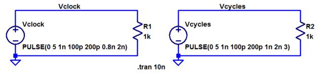
6. Suppose you are doing a sim where you need a clock signal operating at 10 MHz that oscillates between 0 V and 5 V. Assume the duty cycle of the clock is 50% (the clock signal is high [= 5 V] the same amount of time that the clock is low [= 0V]). Assume the rising and falling edges are 1 ns. Show how to implement this clock signal in LTspice. (2 points)
