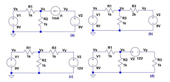
2. Determine the currents and voltages in the following circuit using mesh analysis. Verify your hand calculations using LTspice. (4 points)
