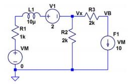
5. Calculate Vout in the following circuit. Verify your calculations using LTspice. (2 points)
