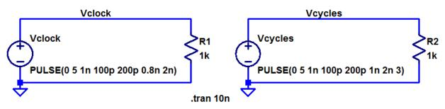
6. Suppose you are doing a sim where you need a clock signal operating at 10 MHz that oscillates between 0 V and 5 V. Assume the duty cycle of the clock is 50% (the clock signal is high [= 5 V] the same amount of time that the clock is low [= 0V]). Assume the rising and falling edges are 1 ns. Show how to implement this clock signal in LTspice. (2 points)
