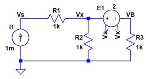
3. Find Vout in the following circuit. For all intents and purposes you can assume the gain of the VCVS is infinite. (3 points)
