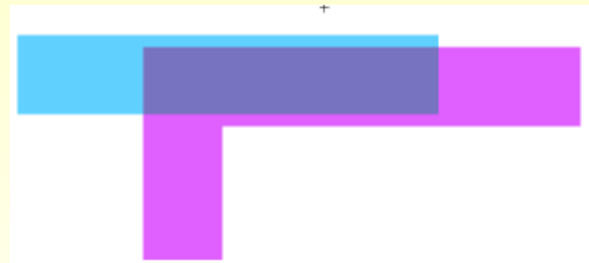
Overestimation : Simple Overlap capacitance
