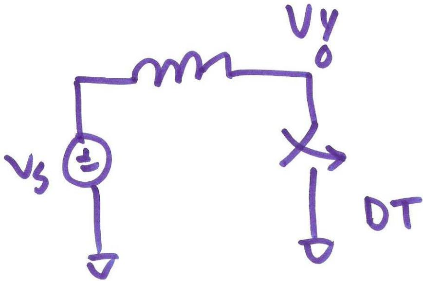
$$\begin{aligned}\Delta i_L &= DT \cdot \frac{v_s}{L} \\ &= (1-D)T \cdot \frac{v_s - v_y}{L}\end{aligned}$$
